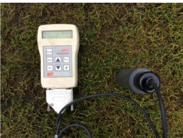
Figure 5: The playing surface is particularly water retentive due to poor infiltration/percolation, recording a value of 41% on the day.
