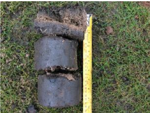
Figure 3: At the wetter, rear of 5 th teeing platform the compaction of the constructed layers is evident which is restricting root development and water percolation.
