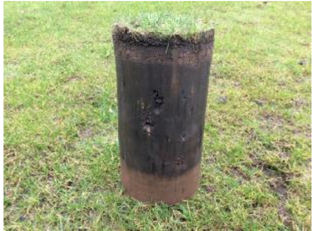
Figure 2: The soil profile taken from the relatively dry front section of the 5 th tee reveals the composition of materials used.
